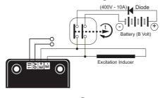
The battery must be isolated from the mass.
