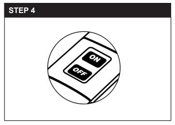
Push ON to activate Start cycle. Push OFF to activate Stop and Cooldown cycle.
