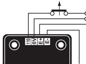
The exciter is switched off by disconnecting the A.V.R. power supply (1 wire - 0 or 110V). Contact rating: 16A - 250V AC
