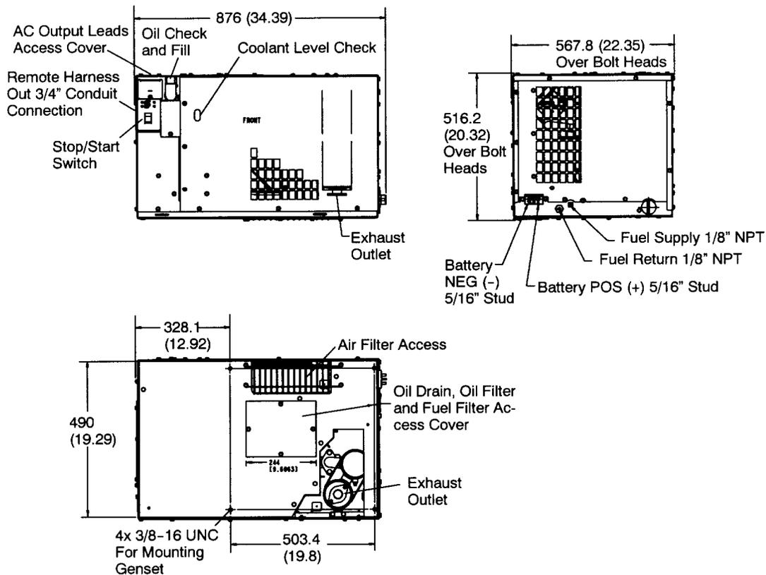
**Note:** This outline drawing is provided for general reference only and is not intended for design or installation. For more information see Operation and Installation manuals or obtain drawing 500-3634 and wiring diagram from your distributor/dealer.
