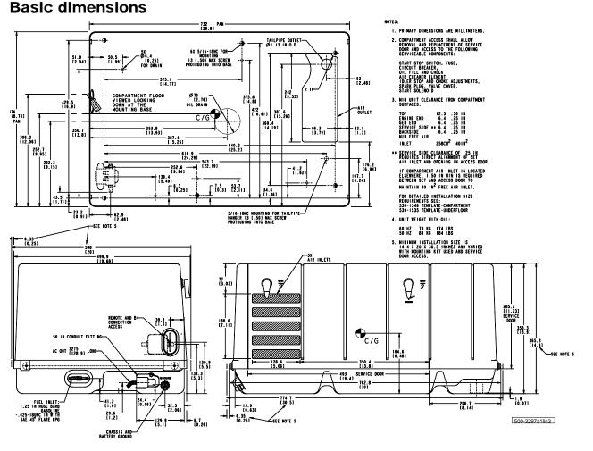
**Note:** This outline drawing is provided for general reference only and is not intended for design or installation. For more information see Operation and Installation manuals or obtain 500-3297 drawing and wiring diagram from your distributor/dealer.
